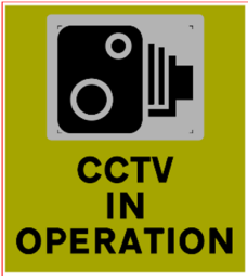
Figure 6 Small standard sign for vehicles or other equipment fitted with CCTV
